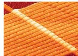
Fig.5.2. Nano-sized Memristor
