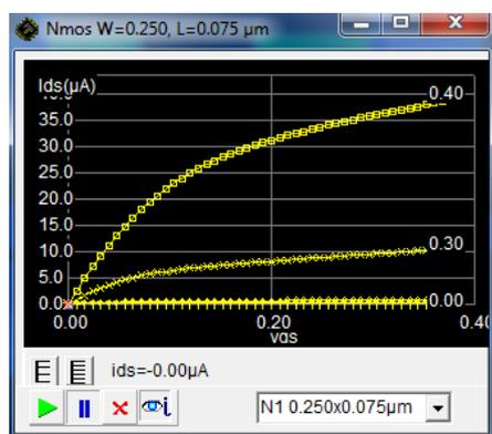
Fig.3.2. Characteristics curve for N1 transistor of 6-T SRAM cell
