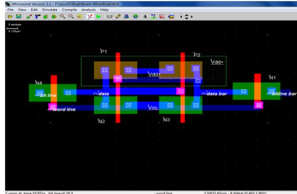
Fig.2.3. Layout design of the 6 transistor static RAM memory cell
