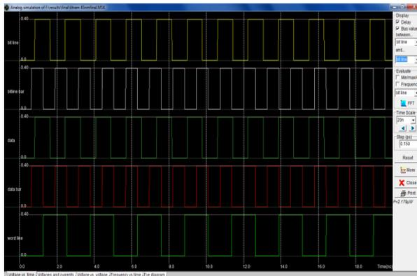
Fig.3.1. Simulation for the 6T static RAM memory
